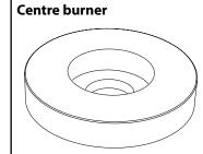
If you are converting to LP Gas the burner ring in the centre burner must be changed for the large ring in the conversion kit.
